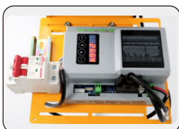
PWM variable frequency servo controller board
